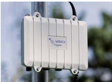
Access can be granted from each WiBACK node via ethernet, or a connected access network (WiFi, WiMAX, GSM, 3G, 4G, etc.)
